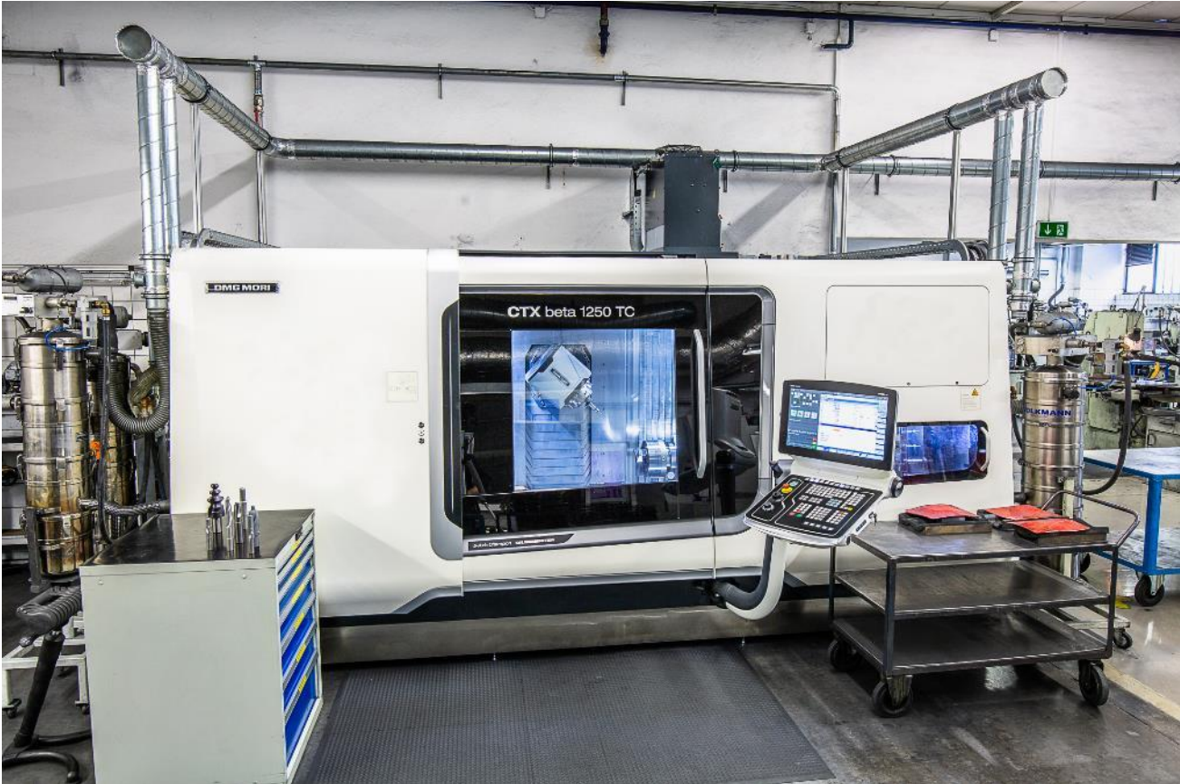
Abb. 1: Flexibility for batch size 1: Thanks to special clamping technology, the turning-milling center from DMG offers new possibilities for machining complex, chalk-like preforms.
