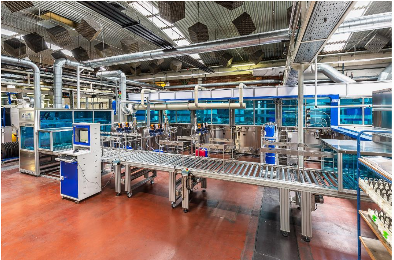
Fig. 1: The automated multi-chamber cleaning system offers flexibility at the highest level: Cleaning processes may now be adapted to individual requirements.
