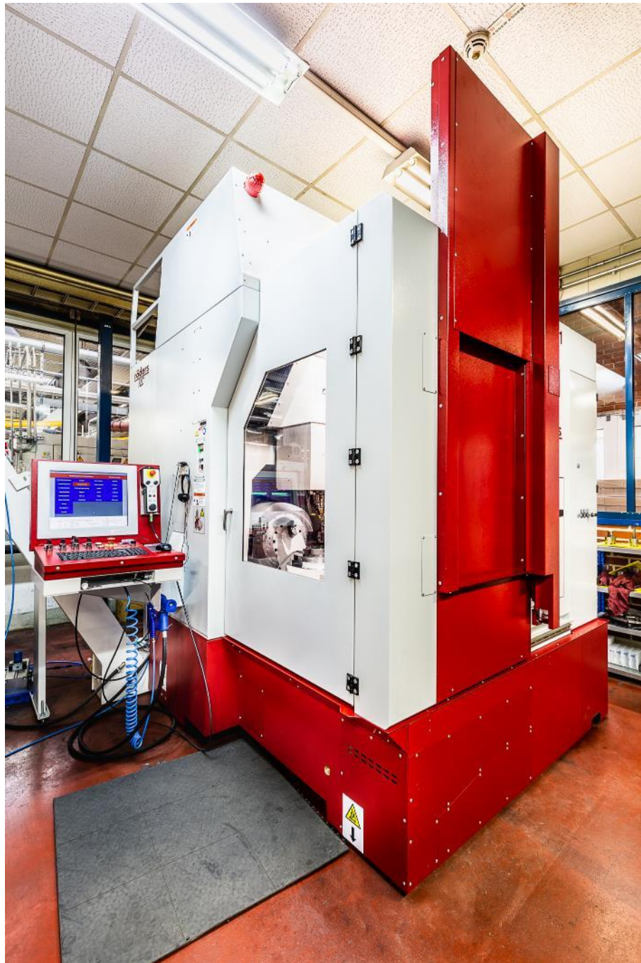
Fig. 1: Thanks to a new technology, carbide pressing tools may now also be milled. The 5-axes Rödgers milling machine for high-performance milling, grinding and inspecting.
