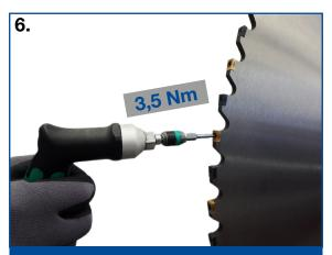
■ Tighten the screw with a torque of 3.5 Nm
