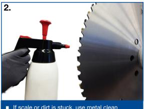
■ If scale or dirt is stuck, use metal clean
