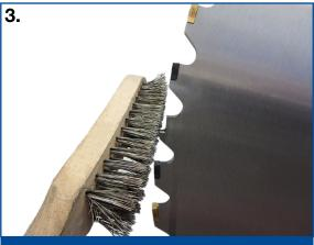
■ Carefully remove any dirt from the plate seat with a copper brush
